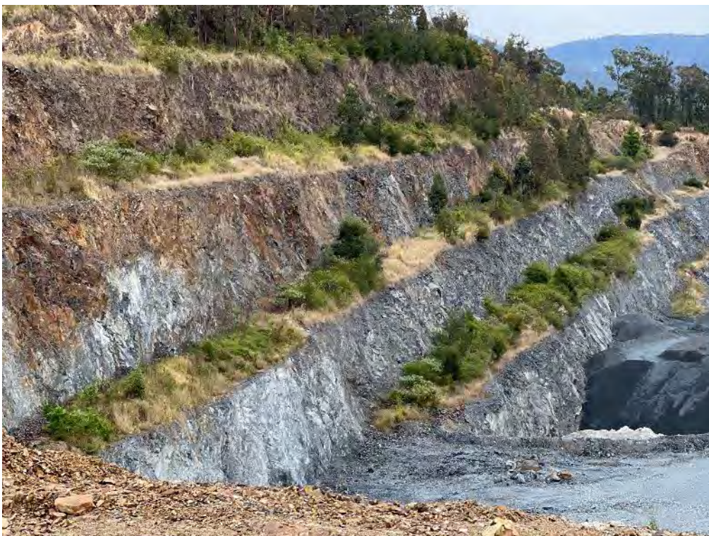
Plate 10: OB2 showing the revegetation of the southern benches in the Active Pit Area
