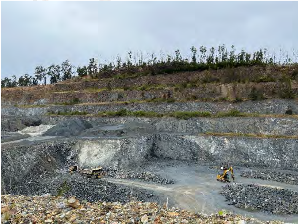
Plate 11: OB3 showing the revegetation of the southern benches in the Active Pit area
