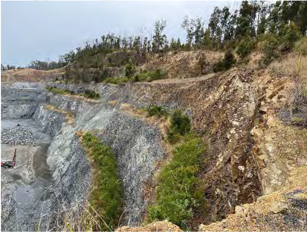
Plate 9: OB4 showing the eastern Active Pit Area Benches. Note the unstable rock face at the right
